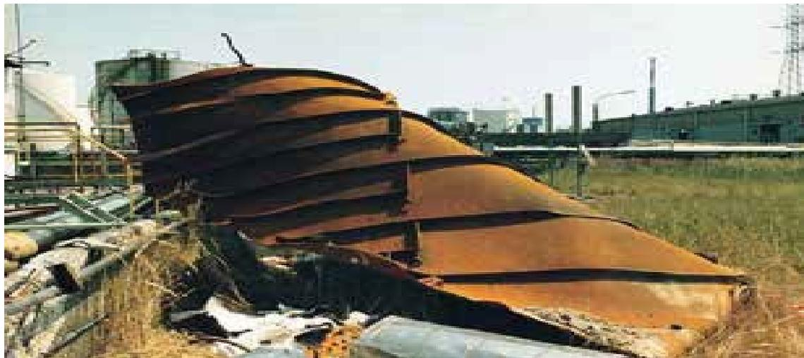
***Ethylene Oxide Leak Under Insulation Results in Tower Explosion***
