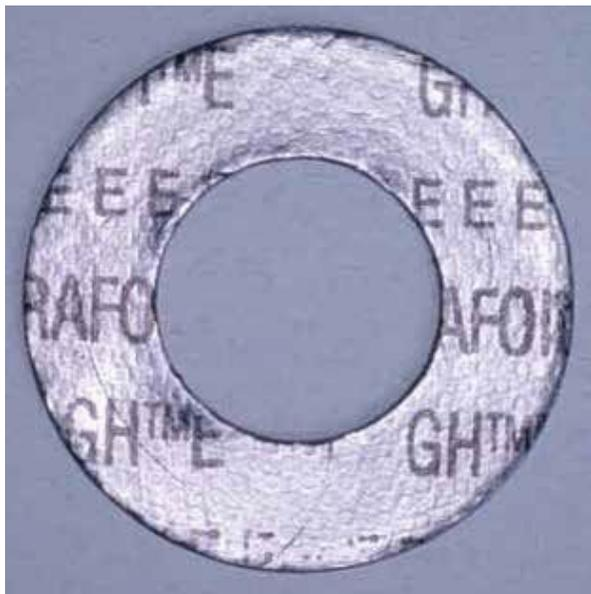
If a laminated gasket is used, it is important to specify a tang stainless steel sheet rather than flat stainless-steel sheet. Tests have shown that EO will attack some adhesives that are used to bond flexible graphite to flat stainless-steel sheet (Figure6.8).
