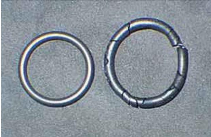
Figure 6.10 A & B Illustrates degradation of FFKM attack over time in service
