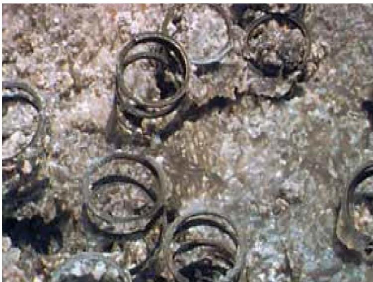
Figure 5.23 Filter Case after Runaway Polymerization
