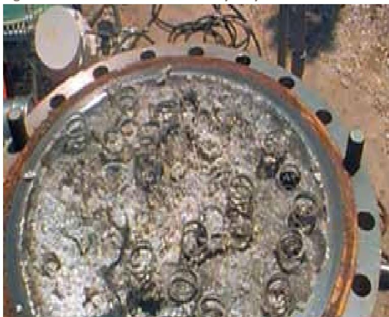
Figure 5.22 Filter Case after Runaway Polymerization
